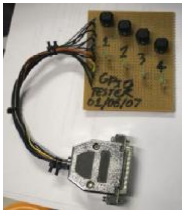
Example Hardware GPIO test rig, featuring 4 trigger buttons, and 4 Output L.E.D. tally lights
